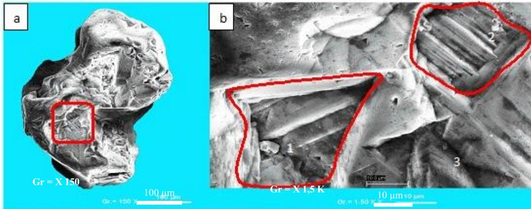
**Fig. 16. Sand grain with many traces of shocks with dissolution figures in Aforenou (Ghana)**
