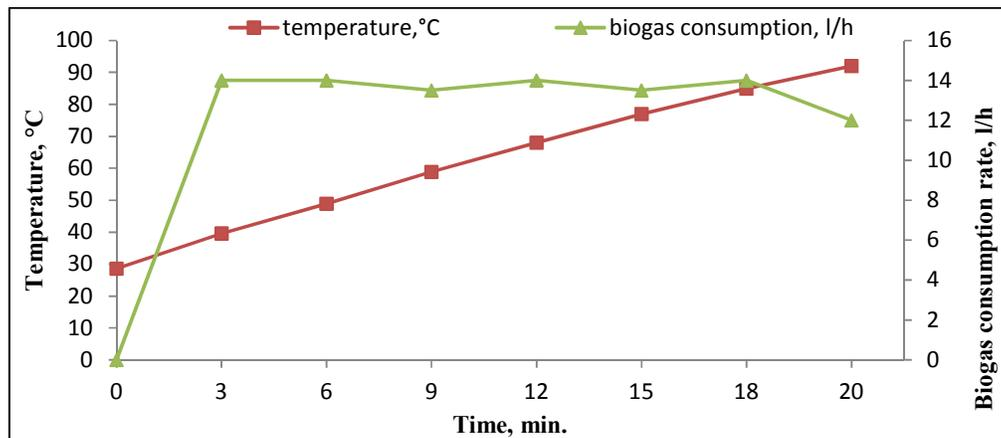
Fig. 1. Variation of temperature and biogas consumption rate (l/h) with respect to time (min.) during water boiling test
