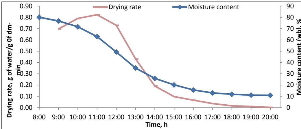
Fig. 3. Variation of moisture content (wb) % and drying rate with respect to time (h) during full load test at 2 m/s
