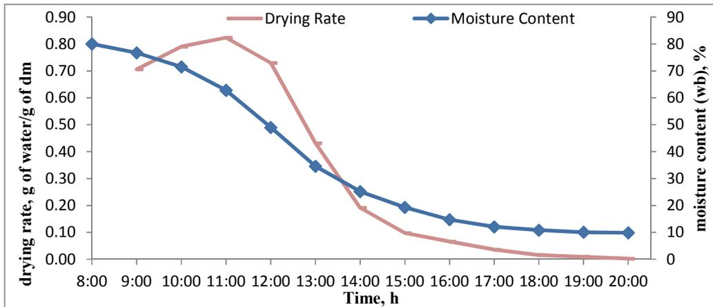
Fig. 4. Variation of moisture content (wb) % and drying rate with respect to time (h) during full load test at 2.5 m/s
