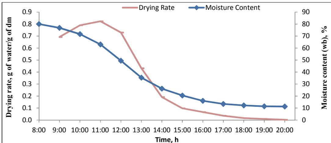
Fig. 5. Variation of moisture content (wb) % and drying rate with respect to time (h) during full load test at 3.0 m/s
