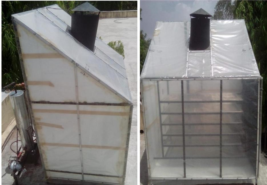
**Plate 1. Developed solar-biogas hybrid greenhouse dryer**
