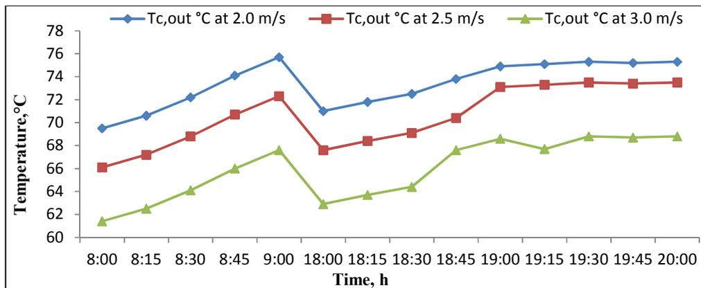
Fig. 2. Variation of air temperature (°C) for different air velocities (m/s) with respect to time (h) at outlet of air heater
