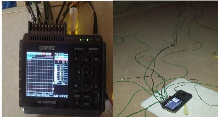
**Fig. 6.** Image of midi data logger **LOGGER GL220** used in this study
