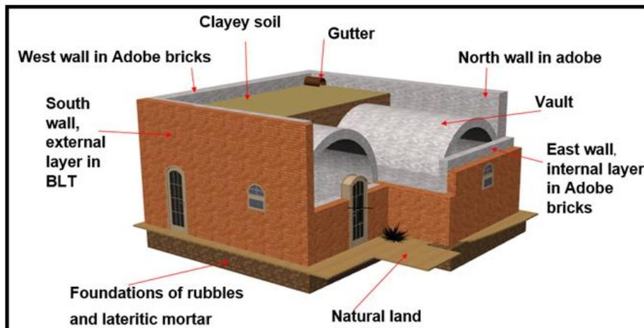
Fig. 1(c). Design 3D of the study house emphasizing the vaults and the walls layers
