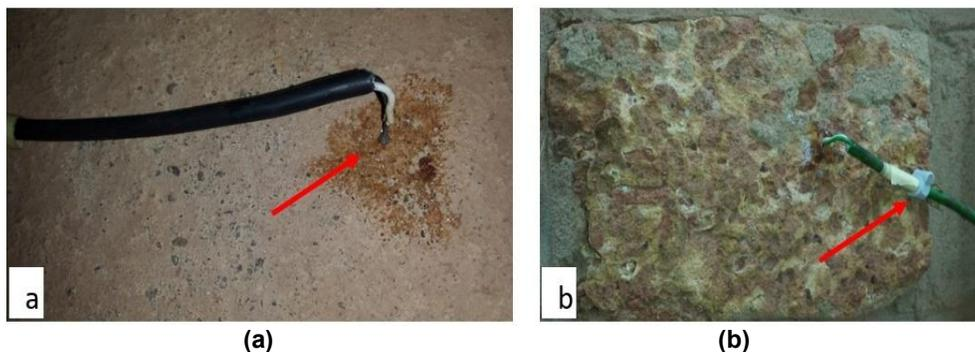
**Fig. 7.** (a) Thermocouple placed with the use of thermal grease; (b) Thermocouple immobilized with a clip
