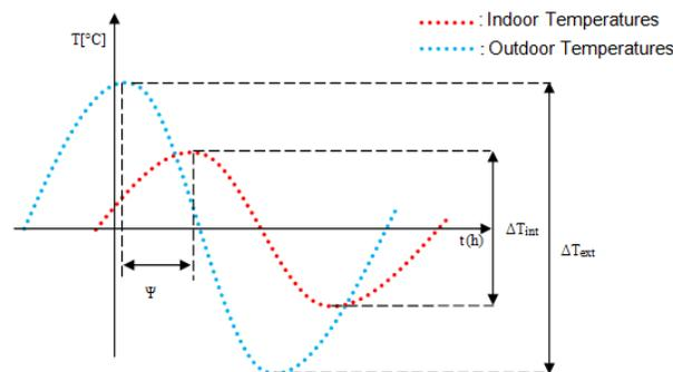
**Fig. 5. Illustration of thermal time lag  $\Psi$ , decrement factor and thermal amplitudes  $\Delta T$**
