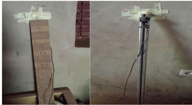
Fig. 9. Images of thermocouples immobilized with wooden and metal tube supports
