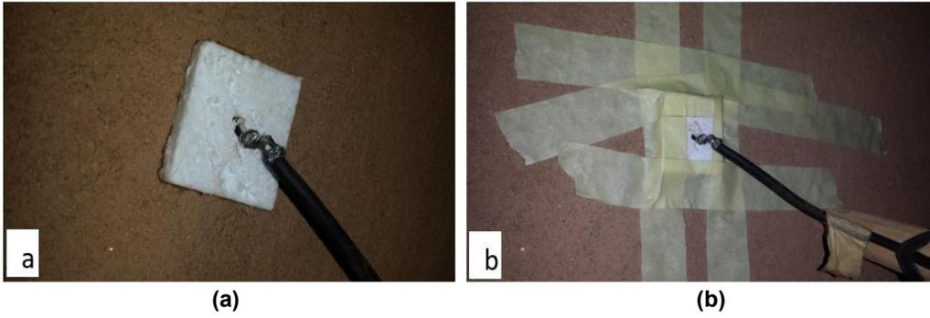
Fig. 8. (a). Thermocouple image placed and insulated with polystyrene; (b) Thermocouple image placed and insulated with polystyrene and reinforced with sticky paper
