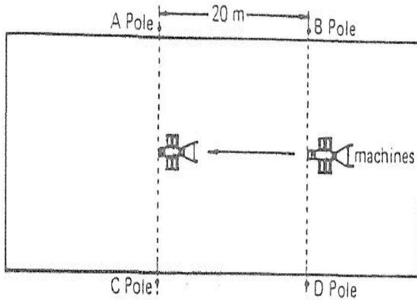
**Fig. 4. Field measurement of operating speed**
