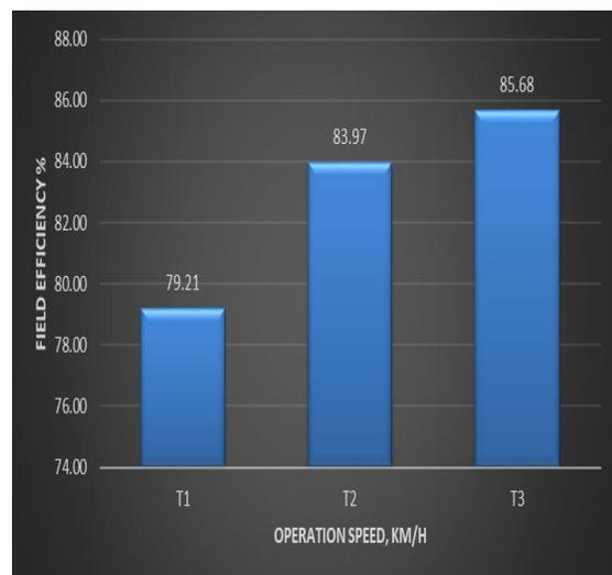
Fig. 11. Graphical representation of Field efficiency Vs speed of operation
