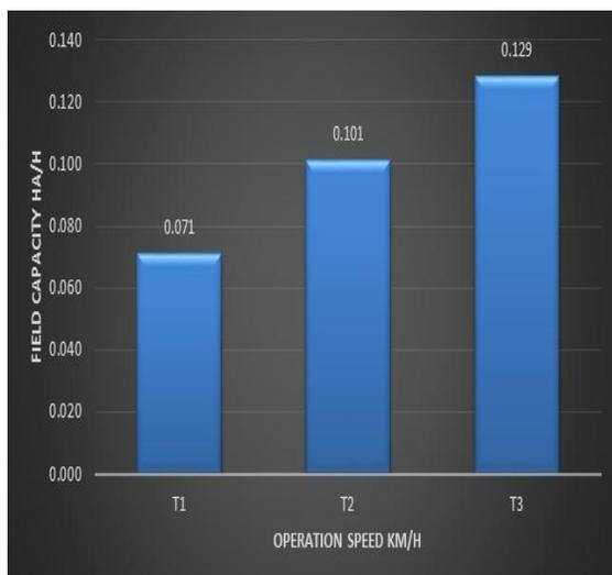
Fig. 10. Graphical representation of field capacity Vs speed of operation
